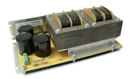
The PSA80V4A-1 power supply has a single 80V output, a voltage input of 115 or 220VAC, and power capabilities of up to 320 watts. With an unregulated output and a size of 8.30" x 4.25" x 2.81" and dual mounting position "L Bracket," the PSA80V4A-1 can be mounted just about anywhere. The PKG-342-MBC12-PS-CBL includes two wires for powering the MBC12101.
